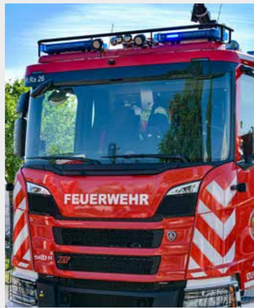
The DBS 850 in divided version (650 mm) with two pairs of additional flashers blue and one pair of power flash.
