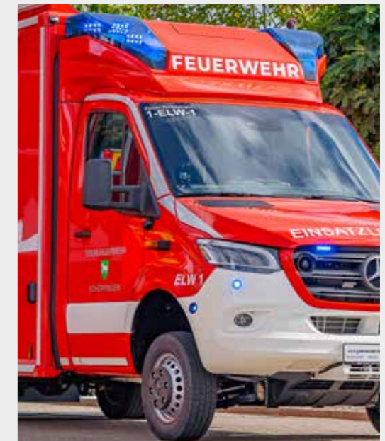
The INTEGRO solution from GSF Sonderfahrzeuge. Shown: a command vehicle (ELW) with box body and all-wheel drive.
