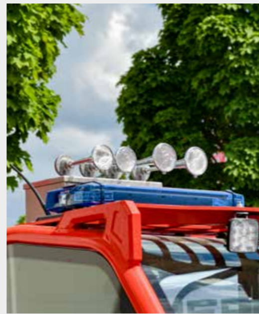
The DBS 850 in full-length version as a special variant (650 mm) mounted on the cab roof of a telescopic handler.
