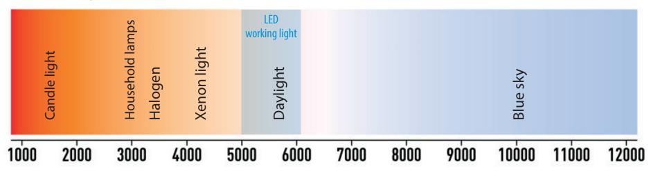
The light colour, also called the colour temperature, is measured in Kelvin. Daylight has a light colour of 5,500 Kelvin. A good LED working light should have a light colour between 5,000 and 6,000 Kelvin. Values that are much higher than this cause human eye fatigue after a long period. The light appears too bright and problems regarding colour reproduction occur.
