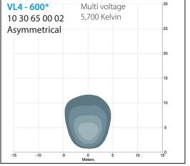
1 Lux 2 Lux 5 Lux 10 Lux
