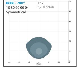
1 Lux 2 Lux 5 Lux 10 Lux 25 Lux 50 Lux
